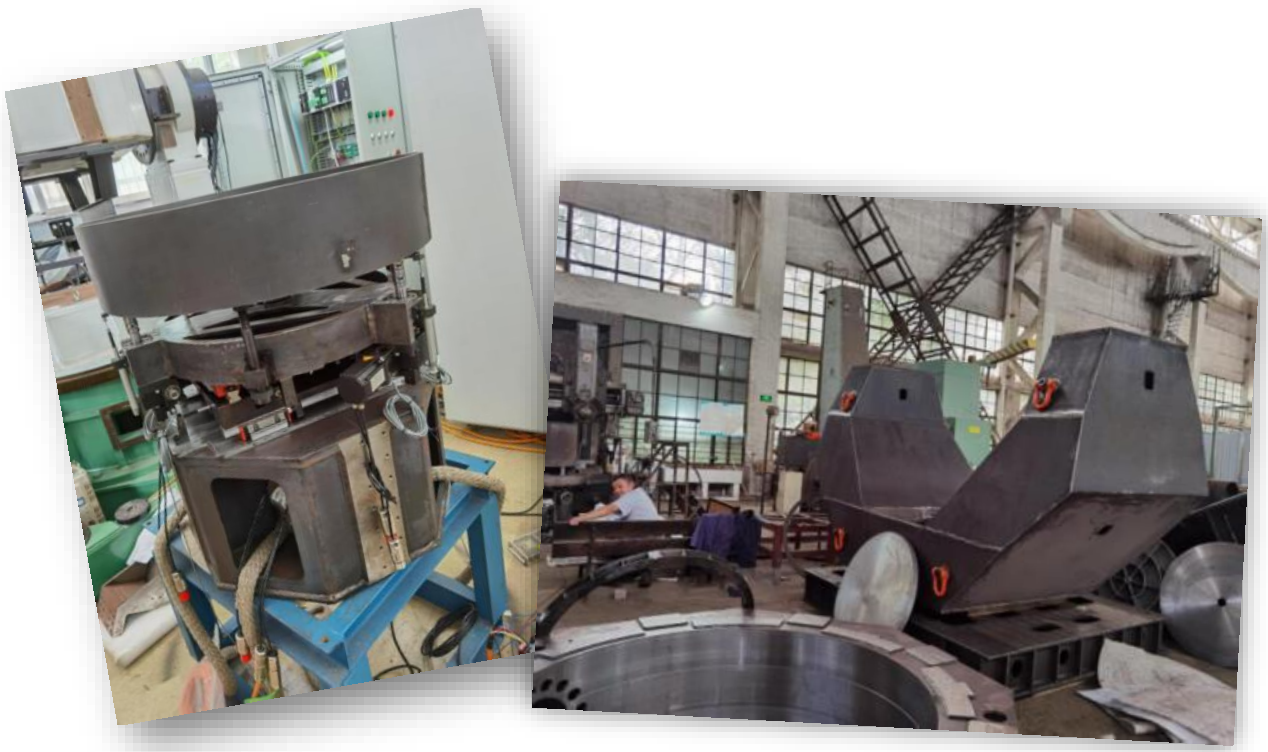
图 3.2: 左: 副镜支撑五维调节机构; 右: 部分机架部件 Left: the 5-dimensional regulating device for secondary mirror support; right: some components of the whole frame structure
